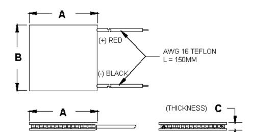
Ceramic Material: Alumina (Al<sub>2</sub>O<sub>3</sub>)
